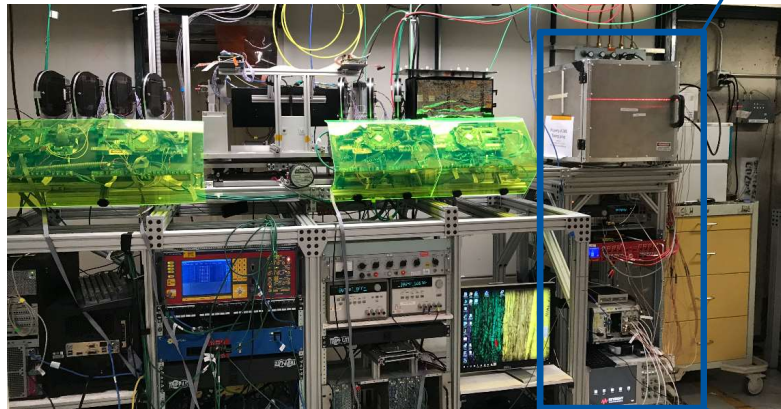
Permanent mechanical structure: ETL cold box can slide in and out of beamline as needed
