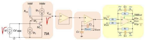
A Transimpedence Amplifier readout scheme
