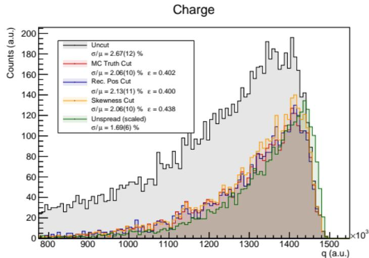
Reduced charge/energy resolution due to lateral events.
