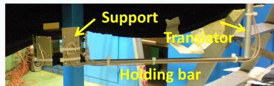
The translation system permits to vary the source distance from the PMT plane in a 0-90 cm range. The rotation, is in a 0-90° degree range allowing the positioning below different PMTs.
