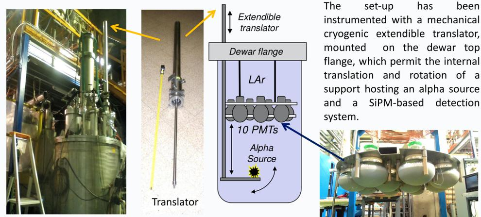
The set-up has been instrumented with a mechanical cryogenic extendible translator, mounted on the dewar top flange, which permit the internal translation and rotation of a support hosting an alpha source and a SiPM-based detection system.
