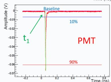
The determination of the delay ( $t_1 - t_0$ ) between the SiPM response and the PMT activation is performed by determining for each event the intersection point between the baseline and the extrapolated line fitting the 10% and 90% of the signal amplitude.
