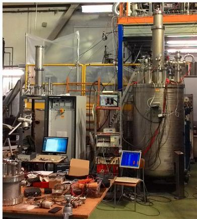
A LAR test facility has been set up at CERN [1] to perform at small scale studies on performances of DAQ and trigger electronics to be installed in larger volume LAR-TPCs, such as ICARUS at FNAL (see M. Diwan *The ICARUS T600 detector as far detector within SBN program* at this conference).
