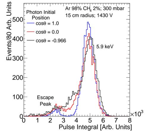
Figure 7: Pulse integral for 5.9 keV photons with an initial radius of 14.5 cm.
