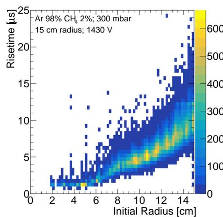
Figure 8: Initial electron radius versus pulse risetime for 2.38 keV electrons with an initial  $\cos\theta > -0.8$ .
