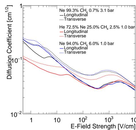
Figure 2: Electron diffusion parameters from Magboltz.
