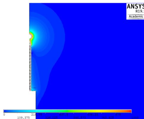
Figure 3: A profile of the electric field near the 2 mm diameter anode in a 30 cm diameter spherical proportional counter, modelled in ANSYS [3].
