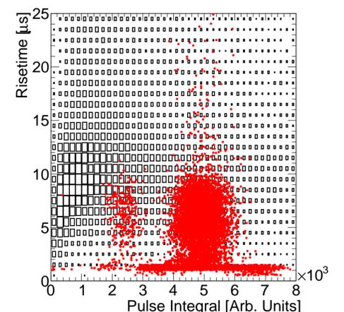
Figure 9: Risetime vs pulse integral for muons incident from a plane above the detector (black) and 5.9 keV photons (red).
