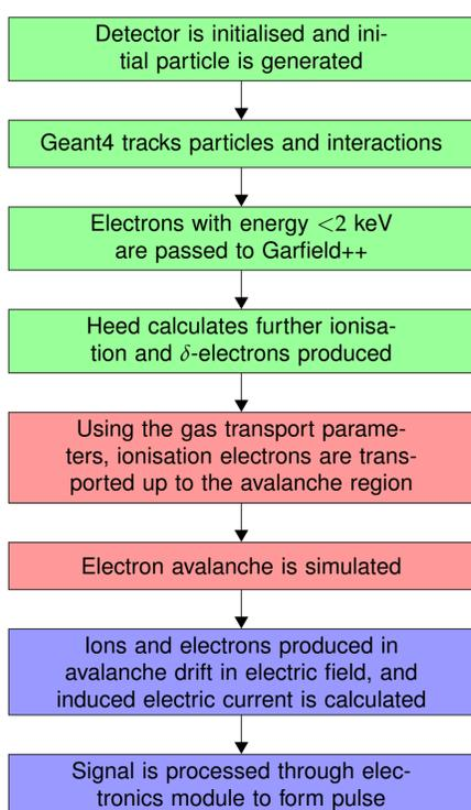
Figure 4: Flow of an event within the simulation framework: Initial interactions in green, electron drift and avalanches in red, and signal calculation in blue.
