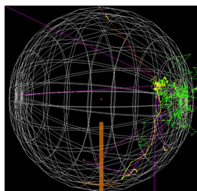
Figure 5: Geant4 visualisation of a muon traversing a spherical proportional counter.
