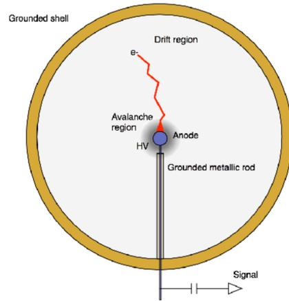
Figure 1: Principle of operation of the spherical proportional counter [3].
