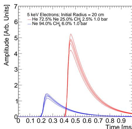
Figure 6: Example readout pulses produced by 5 keV electrons from an initial radius of 20 cm for different gas mixtures.
