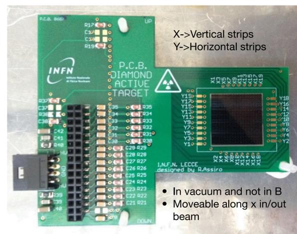
Diamond sensor:  $2 \times 2\text{cm}^2$  area and 100  $\mu\text{m}$  thickness.
