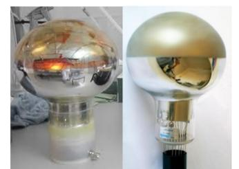
Figure 10: Different PMTs: polish (left) and sandblasted (right).
