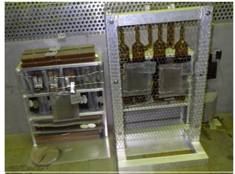
GFRP Samples from KEK, CERN and LBNL set at Co60 Gamma Ray Irradiation Facility at QST Takasai.
