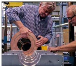
(Left) A view of the PI-Mode Structure (PIMS) cavities, which will accelerate the Linac 4 beam from 100 to 160 MeV. (Right) Mauro Paoluzzi, project leader for the PSB RF overhaul, with one of the FINEMET cavities that will allow more intense beams.
