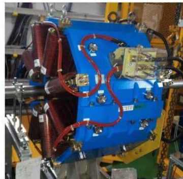
OCTU2 installed in ATF
