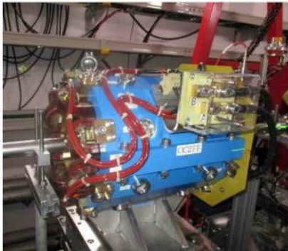
OCTU1 installed in ATF
