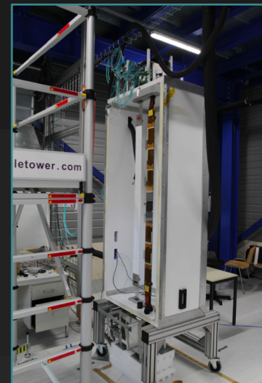
UT slice test with an instrumented stave at CERN
