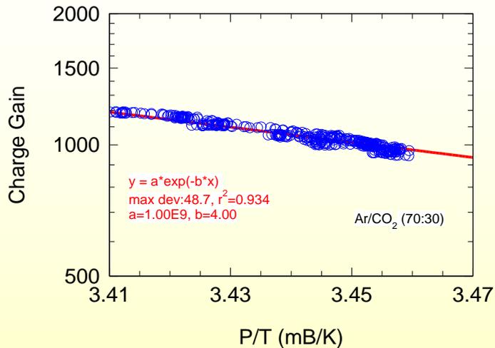
**P/T GAIN SENSITIVITY:** The effective gain of the present GEM over 3 weeks plotted as a function of P/T yielding sensitivity to 4.0 K/mB. This is over two times larger than the P/T sensitivity of a 50  $\mu$ m GEM. Assuming that P is roughly constant at around 1000 mB and allowing for maximum temperature excursion of  $\pm 5$   $^{\circ}$ C from 20  $^{\circ}$ C would result in a maximum gain excursion of 22.9 %.
