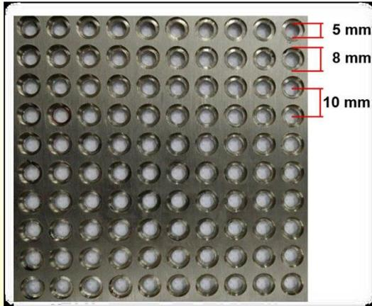
A stainless steel mask, with an array of 100 holes. Each hole acted as support for the colimated  $^{55}\text{Fe}$  source.
