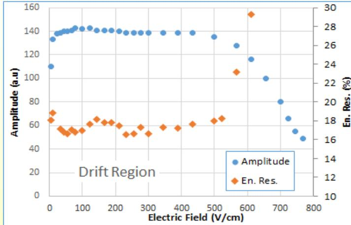
Double GEM Cascade electric field optimization was done in pure Krypton with a discrete  $^{55}\text{Fe}$  source. Results show an improved energy resolution and requirement for lower electric fields to operate the detector.
