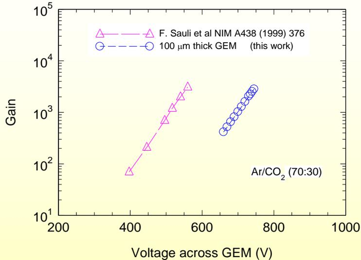
**SINGLE:** Charge gain characteristics of the single GEM\_100 using Ar (70%)-CO<sub>2</sub>(30%) gas mixture. In order to compare the gain response with 50 μm thick GEM, data from elsewhere [Sauli et al 1999] is included for comparison.
