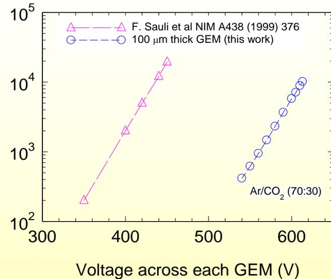
**DOUBLE:** Charge gain characteristics of the double GEM\_100 configuration using Ar (70%)-CO<sub>2</sub>(30%) gas mixture. Uppermost charge gains for 50 μm thick and 100 μm thick GEM are of the same order of magnitude.
