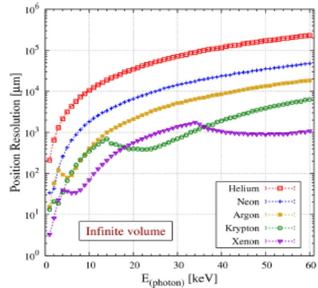
Position Resolution in our system is dominated by SNR (for lower energies) and by the range of the photo-electron in the gas mixture used.
