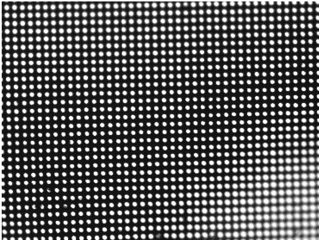
Mesh 45/20 on 10 \mu\text{m} aluminum foil
