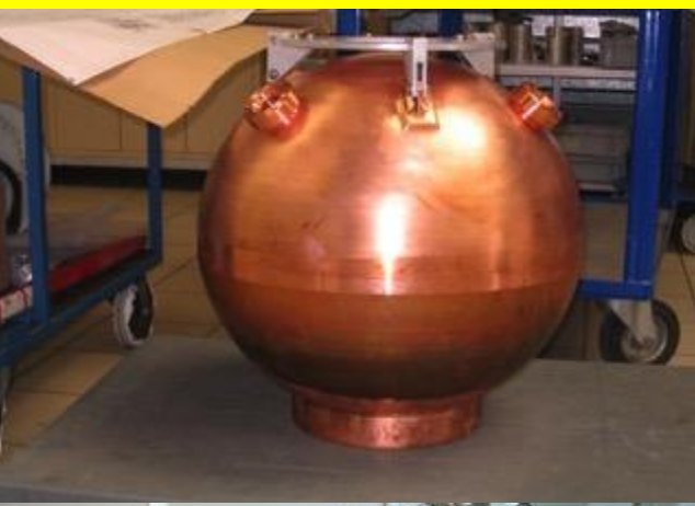
Low background detector d=60 cm p=10 bar
