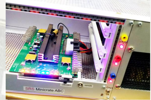
New power access panel and Status LEDs
