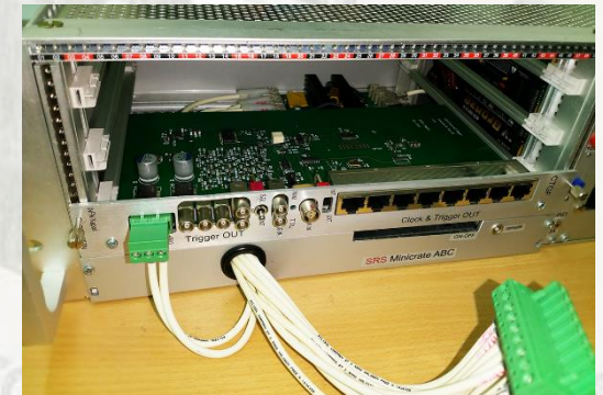
CTF slot and CTF power connector
