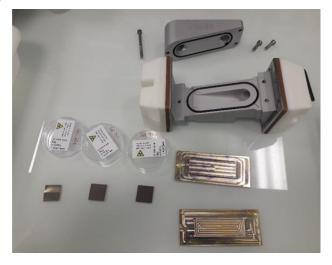
Irradiation: MAY 28 2019 proton beam 15mn -E=60MeV  $-20\mu$ A sur cible  $-5\mu$ A\*h integrated
