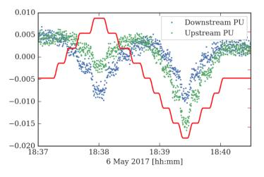
Vertical centering with 3 pilot LHC bunches and orbit vertical bump (steps of 0.5mm)
