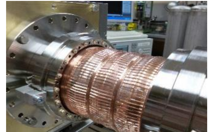
Prototyping and mechanical and RF tests of the deformable RF bridge
