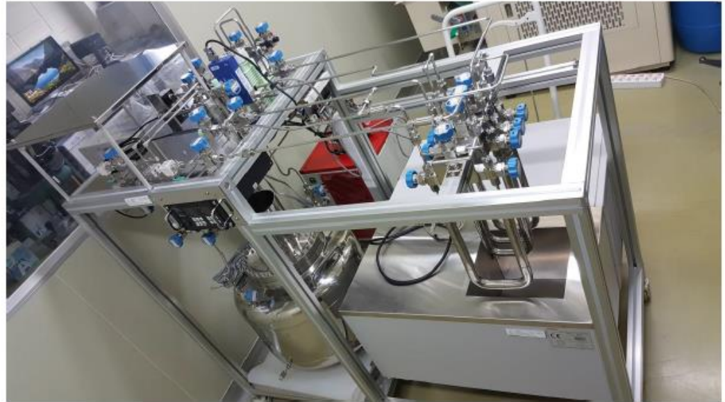
Assembled radon measurement device at SNU
