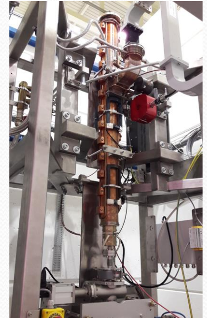
9+ MeV/0.2 mA electron linac Installed at CERN in 2017
