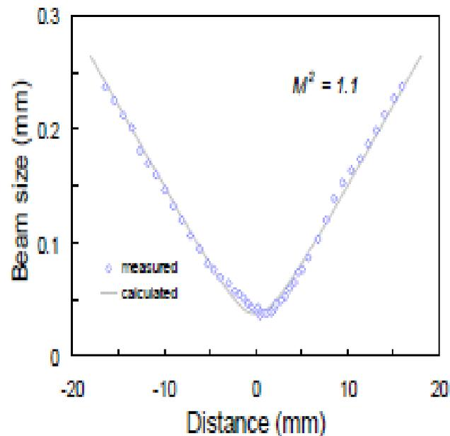
*Measured beam size versus propagation distance through a beam focus. The calculated curve shows the dependence for a Gaussian beam with the indicated  $M^2$  value.*
