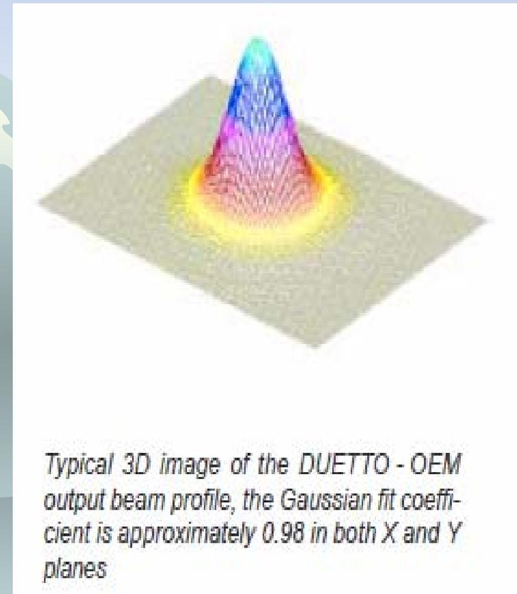
*Typical 3D image of the DUETTO - OEM output beam profile, the Gaussian fit coefficient is approximately 0.98 in both X and Y planes*
