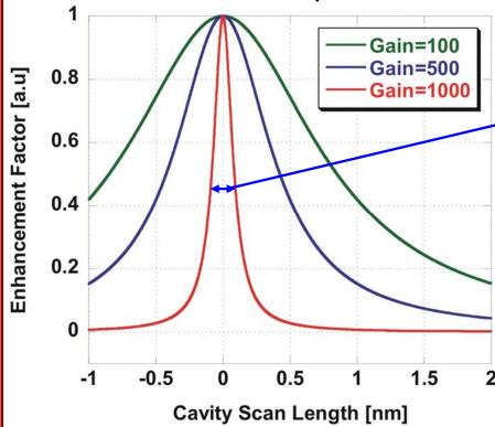
We should control the resonator length <0.1nm
