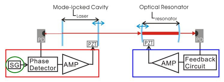
Mode-locked laser PLL (Phase Locked Loop)
