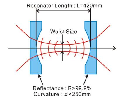
At first, we develop the resonator finesse to maximize the number of x-rays.
