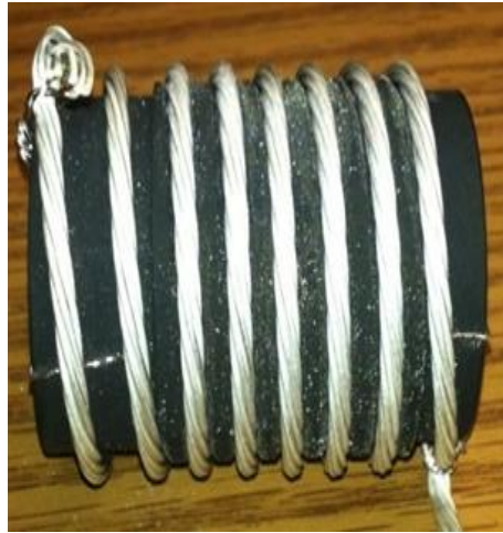
FNAL Breakthrough in HTS cables
