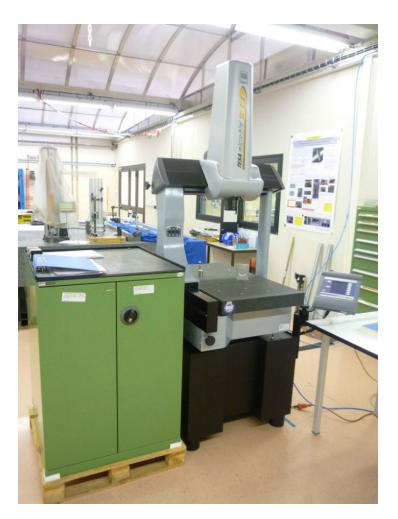
Measurement volume: 460 x 510 x 420mm Precision:  $^{\sim}$  10  $\mu$ m (depends on application and operator)
