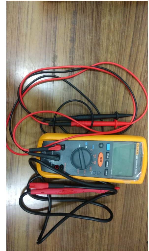
Megger for Insulation test
