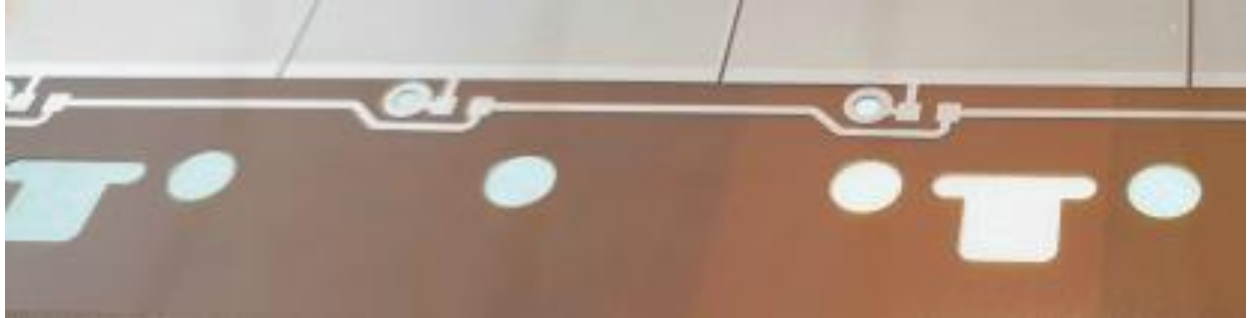
1. Shape of the resistor pads before assembly.
