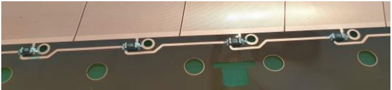
2. Shape of the resistor pads after assembly.
