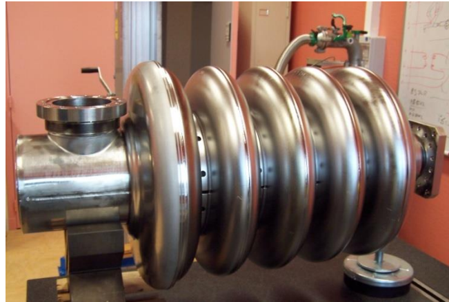
INFN & CEA 704 MHz elliptical SC cavities
