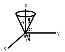
Consider a particle rolling due to gravity in a frictionless cone. The cone's opening angle  $\alpha$  places a constraint on the coordinates  $\tan \alpha = \sqrt{x^2 + y^2}/z$ . It is convenient to write the kinetic and potential energies in cylindrical coordinates
