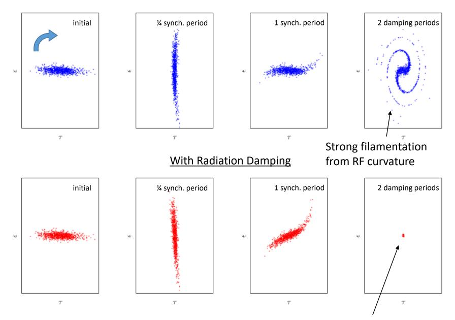
Injected beam dimensions reduce in both au and  $\epsilon$
