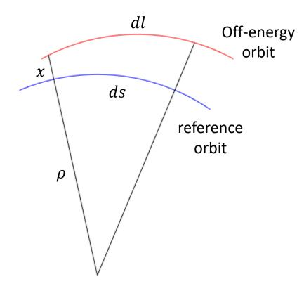
From the bend angle, the difference in path length between the on and off-momentum orbits is
