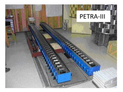
Damping wigglers can be one way of increasing the synchrotron radiation emission.
