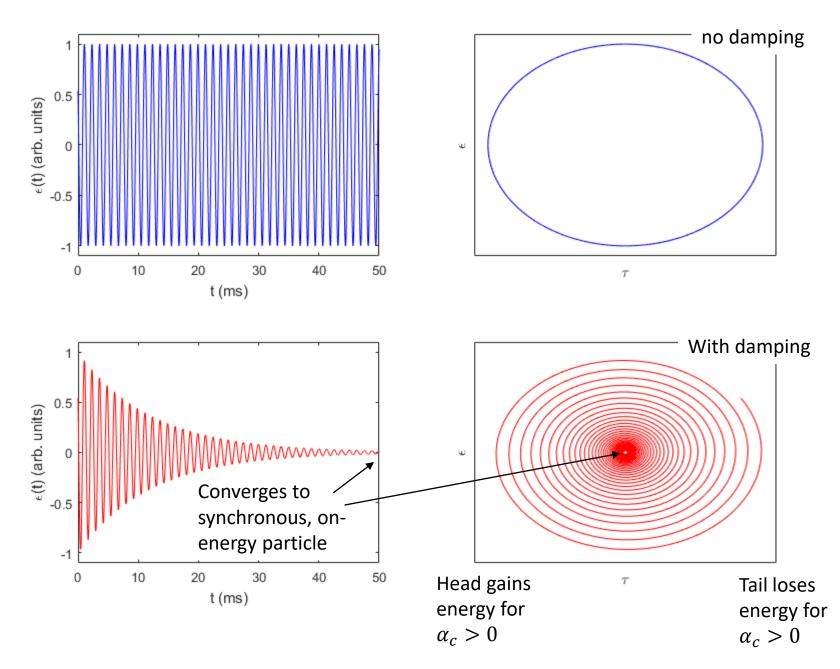
From the previous analysis, the origin of the damping can be seen to have come from the change in energy loss per turn with energy:
