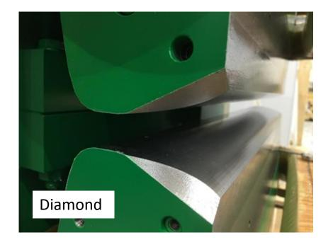
Combined-function bending magnets have both a main dipole field for steering the beam, with a gradient super-imposed on top.
