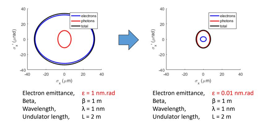
Existing rings already operate close to the diffraction limit in the vertical plane. The challenge is to reduce the horizontal beam size / divergence.
