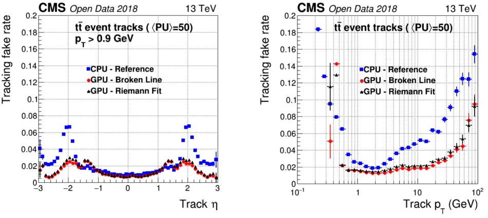
Track reconstruction fake rate as a function of reconstructed tracks  $\eta$ ,
