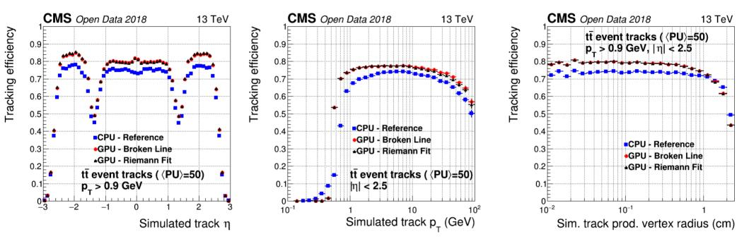
Track reconstruction efficiency as a function of simulated track  $\eta$ ,  $p_T$ , and production vertex radius.
