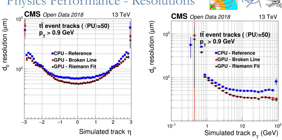
Track resolution of the transverse impact parameter as a function of 25 simulated track  $\eta$  and  $p_T$
