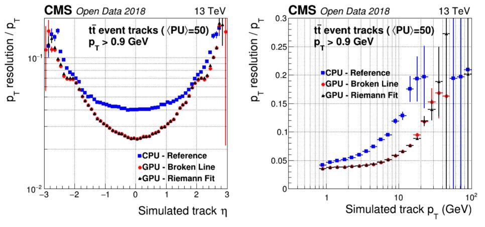
Track reconstruction resolution of  $p_T \, as \, a$  function of simulated track  $\eta \ and \ p_T$
