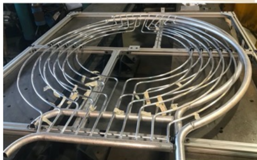
Front Plate: CF+Al Honeycomb+ Source Al Tubing
