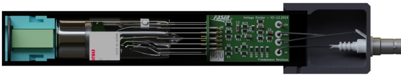
PMT module provides readout pulses A 10 dynode-stage head-on PMT with a cathode diameter of 22 mm
