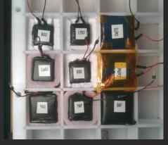
Silicon tracker upstream the prototype: it provides the particle impact position and nuclei charge.
