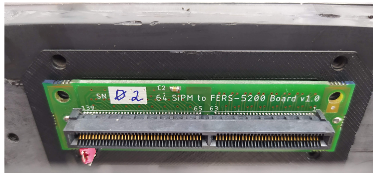
Front end board housing 64 SiPM
