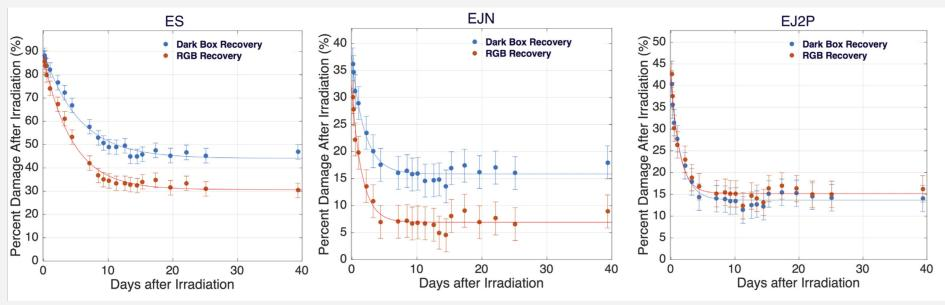
Natural (blue) and RGB LED Stimulated (red) recovery results of lab-produced ES (elastomer scintillator) (left), EJN (Eljen brand EJ-260) (middle) and EJ2P (an over-doped version of EJ-260) (right)
