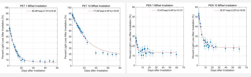
PET (polyethylene terephthalate) recovery results over 21 measurements. 1 MRad Irradiated PET (left), 10 MRad Irradiated PET (right) PEN (polyethylene naphthalate) recovery results over 21 measurements. 1 MRad Irradiated PEN (left), 10 MRad Irradiated PEN (right)
