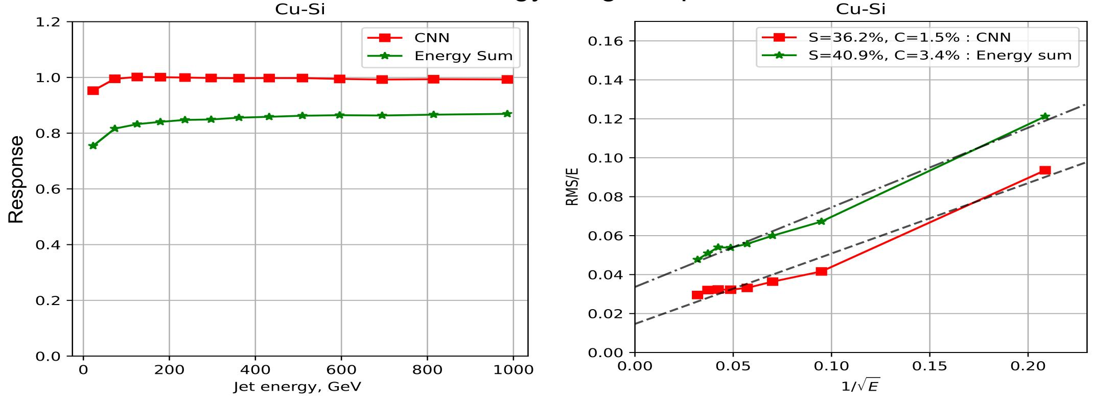
We also tested the CNN trained on single pions for electron energy reconstruction and it maintains good performance comparable to traditional techniques
