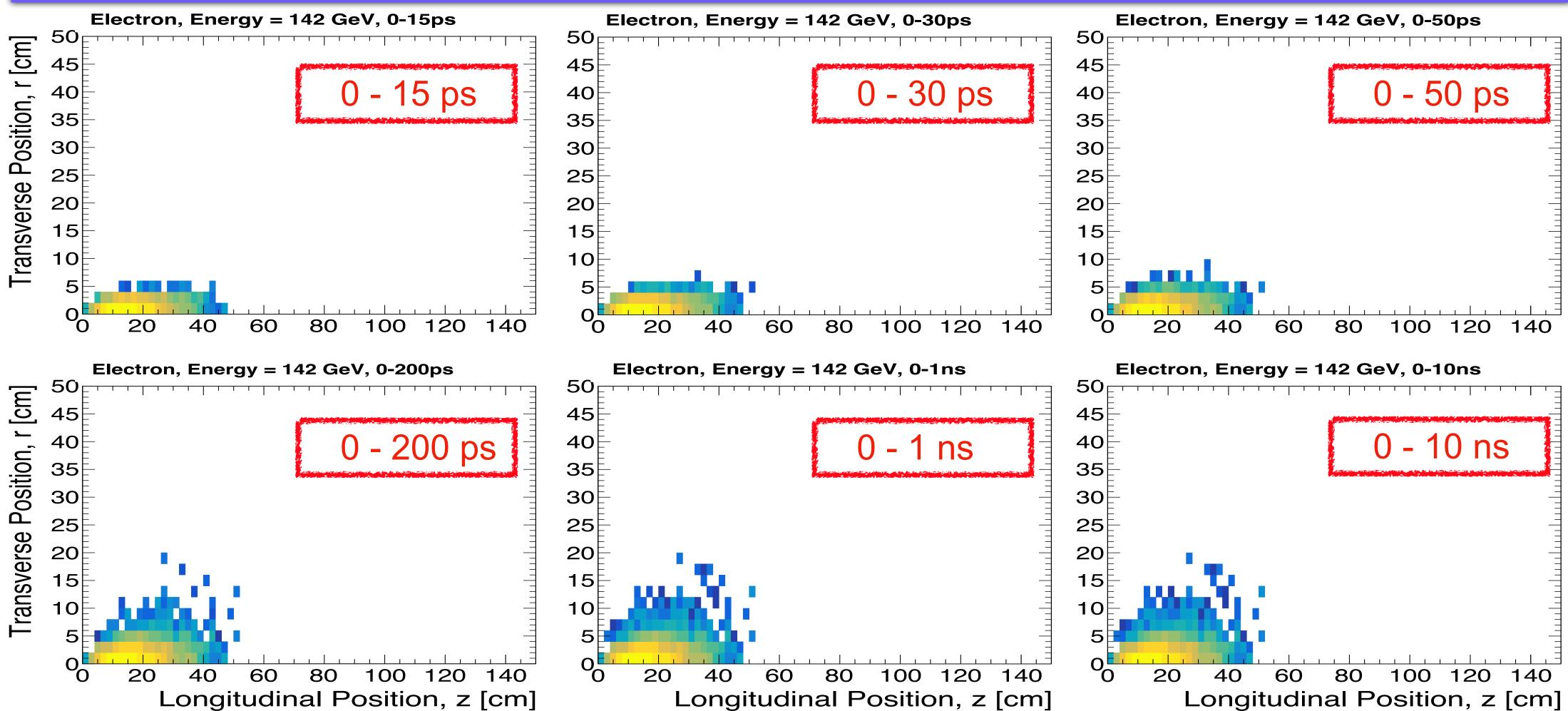
The energy deposits due to a single 142 GeV electron are shown in r - z coordinates where the colors indicate deposited energy. As indicated on top of each each plot, the integration times gradually increase from 0-15 ps (top left) to 0-10 ns (bottom right). Time is 'local', in other words, it is corrected for the travel time,  $t = t_{a} - \frac{z}{c}$ , along z-axis for all particles.
