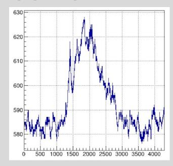
The 127-nm light seems to be coming in bursts. Finer timing analysis is needed. The calculated rate of such pulse trains is ~15 Hz.
