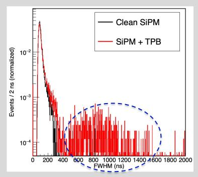
There is a small excess beyond ~500 ns in the SiPM+TPB configuration. The excess also disappears when the SiPM compartment is vented. This is attributed to the 127 nm light.
