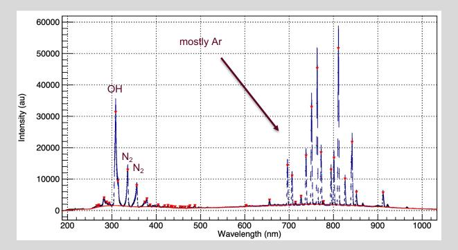
The light source was flushed with argon twice before measurements.
