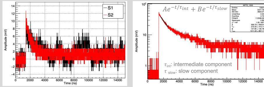
An event display of the two SiPM signals (S1 and S2).
