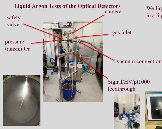
We liquified high purity argon gas in a liquid nitrogen bath.
