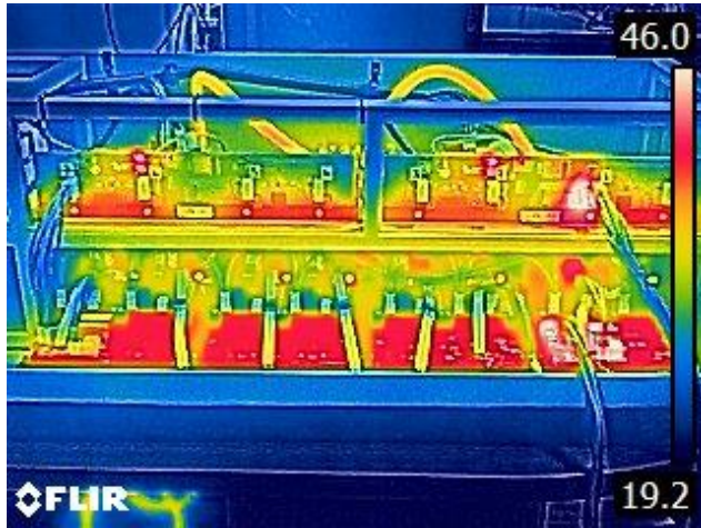
Fig.11 Thermal image of a Burn-in station undertaking burn-in of a Brick
