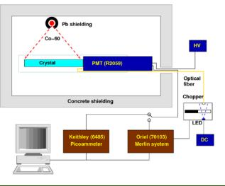
BaF<sub>2</sub> crystals wrapped by Tyvek with an air gap coupling to a Hamamatsu PMT R2059, were irradiated by Co-60 with dose rates of 2 and 23 rad/h
