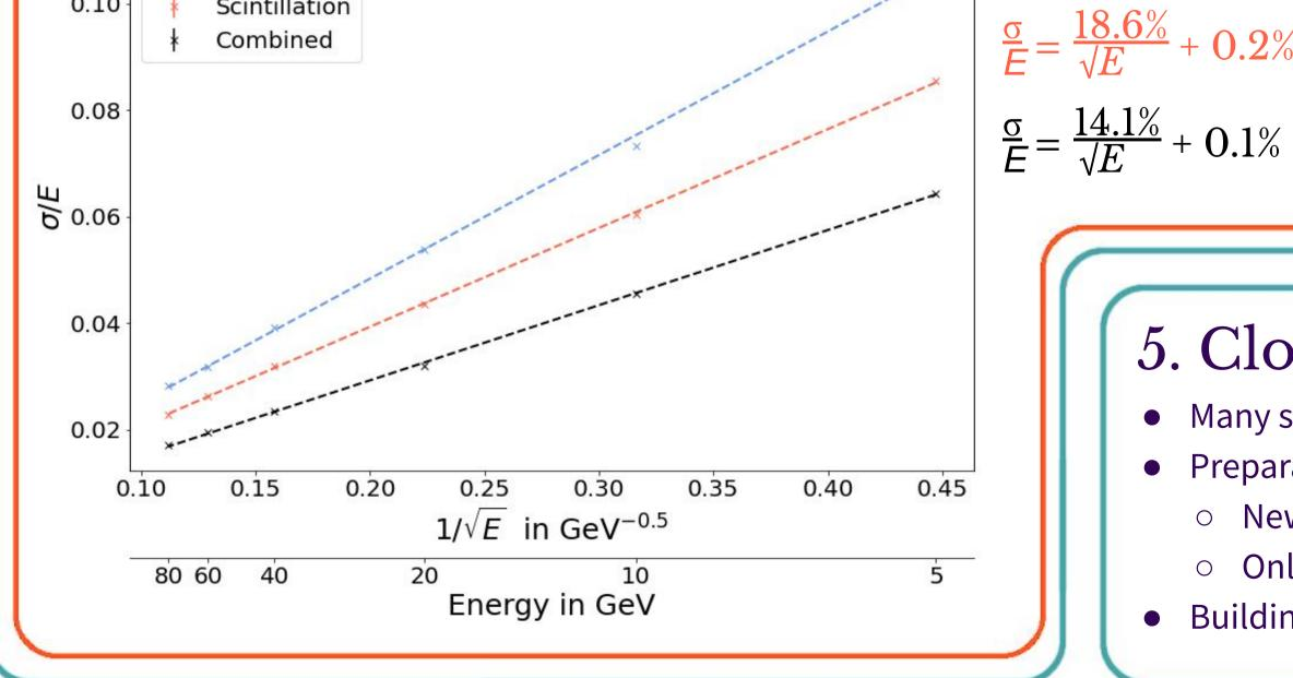
• Combined channel yields an electromagnetic energy resolution of **14.1%**/ $\sqrt{E}$  for this prototype
