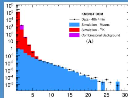
Test of photon counting capabilities and directional sensitivity of DOM
