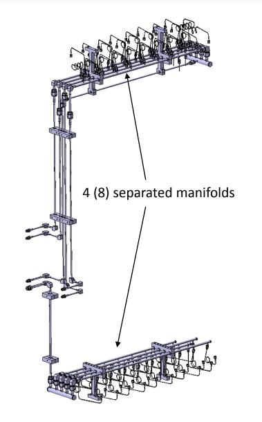
Internal distribution system is divided in 4 manifolds on the top and 4 on the bottom
