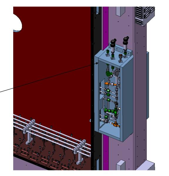
Local box will be attached to the C-frame and in contact with the detector box – no need of insulating pipes between the local box and the detector box. 1. What kind of valves are AV3A20 and AV3C20?
