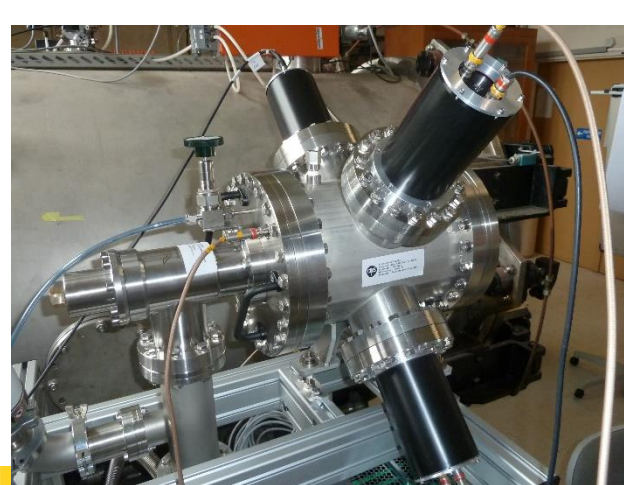
SCALP: Scintillating ionization Chamber for ALpha particle Production in neutron induced reaction
