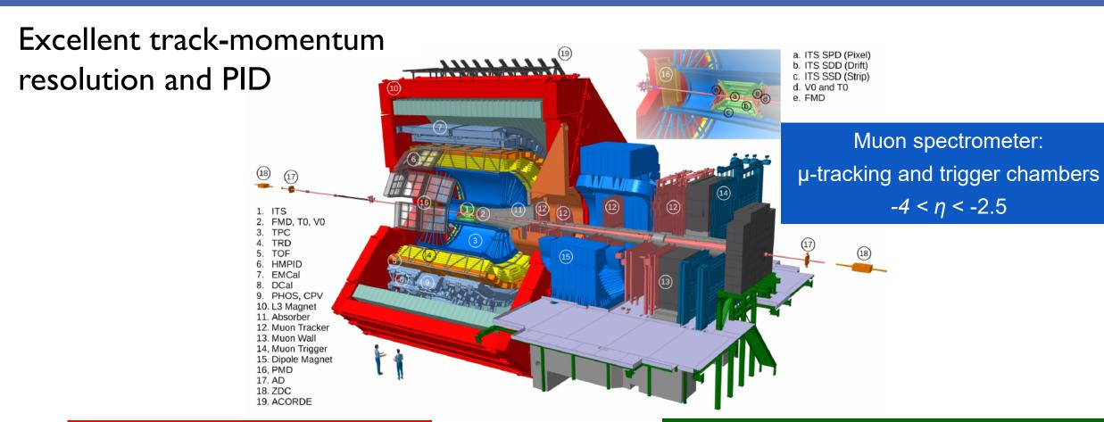
Central barrel: vertexing, tracking, PID, EM calos  $|\eta| < 0.9$
