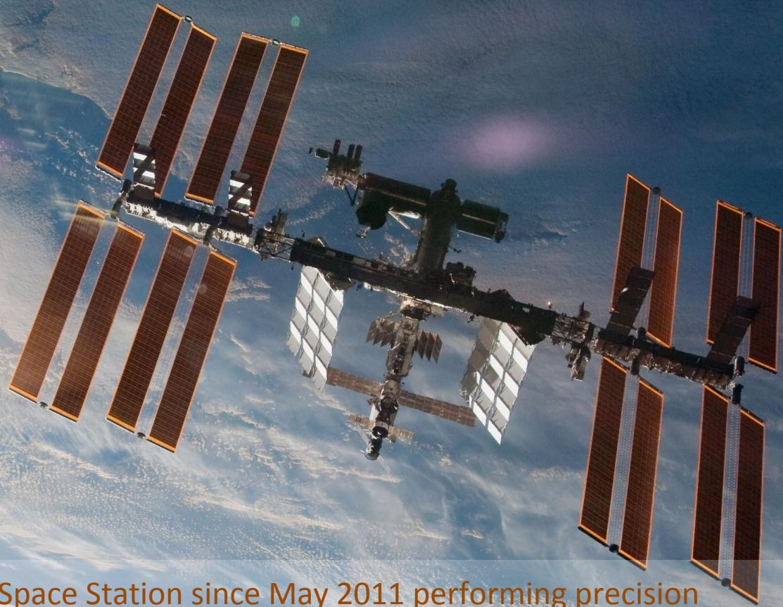
AMS has been operating in the Space Station since May 2011 performing precision measurements of cosmic rays and revealing new details about origin and propagation of all CRs species.
