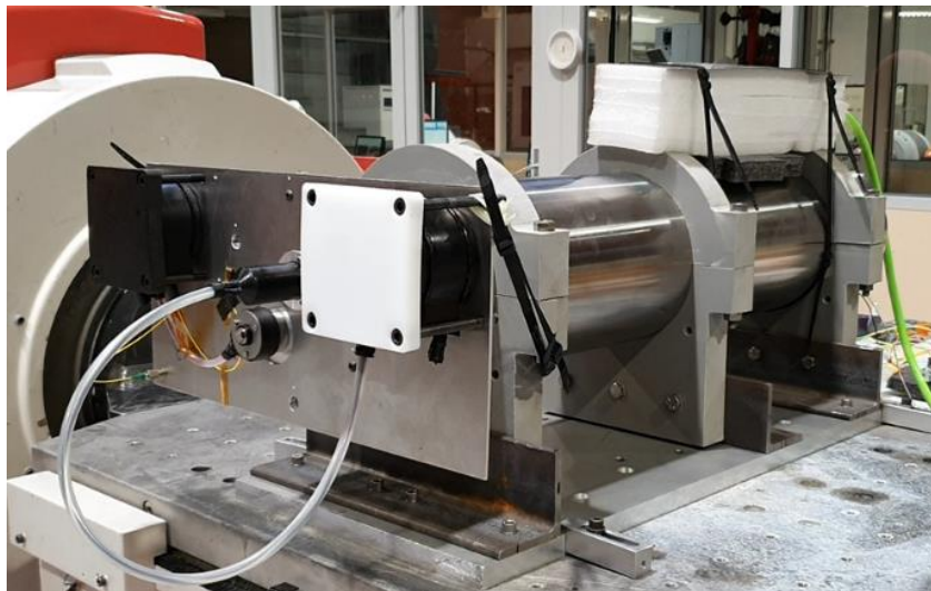
Figure 3: cylinder mounted on the interface plate
