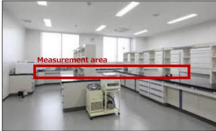
Fig. 2: An image of the visual imager display screen. The area with red square is an indication of the detection area where it is ranged with 16 channels of the MPPC.
