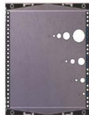
SDD: 2x112 anodes, pitch = 970μm
