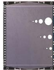
SDD: 2x384 anodes, pitch = 169 \mu m
