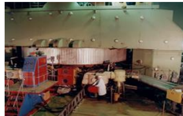
Gatchina cyclotron, 10'000 tons magnet, 1 GeV protons (1957)
